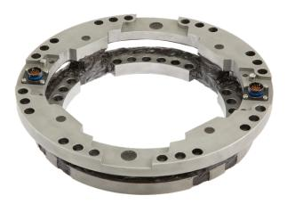
The *LW9.5-HS Wheel Force Transducer (WFT)* is capable of measuring all of the wheel forces and moments on forklift trucks or other heavy vehicles with small wheels. It provides independent output signals for vertical, lateral, and longitudinal forces as well as camber, steer and torque moments. It is completely weatherproof, making it ideal for testing in all conditions. It can also be used to monitor and control laboratory tests.
