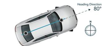
VBOX 3i Dual Antenna is compatible with all existing peripherals, including the Inertial measurement unit which provides a highly accurate speed, distance, heading, and yaw rate measurement for use in ESC testing with a steering robot.
