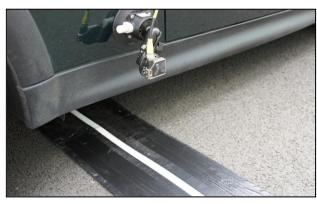
The light barrier is then set facing down towards the ground. This mounting arrangement ensures accurate and consistent strip line detection.
