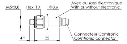
\* Option filetage allongé 10 mm 10 mm lengthened thread option
