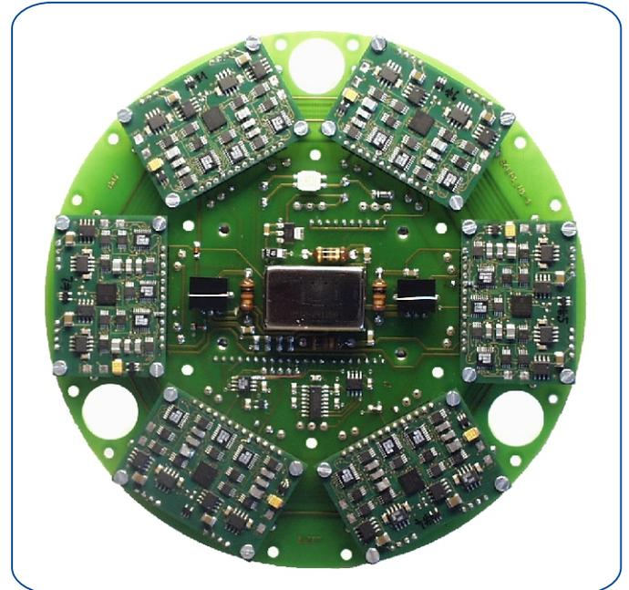
(measuring signals and sensor supplies) can be switched on this converter via a bus. Thus, the signals can be made available as digital signals, too. They are transmitted from the base plate to the PC via an electrically isolated RS232 interface. With the aid of the known SWIFT Terminal program the parametrisation of the PSGC-1 modules is also carried out via the same interface. There is no need to connect the PC during the actual measuring process.
