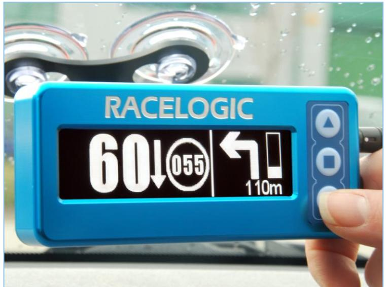
*Above: the speed profiler OLED display is showing a speed of 60km/h, and that the driver must slow to 55km/h. The amount of user deviation permitted from the required speed is adjustable. The speed profiler is also stating that the driver must turn left in 110 meters.*
