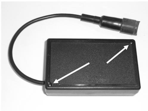
Remove the 2 (two) Phillips screw to access the batteries.
