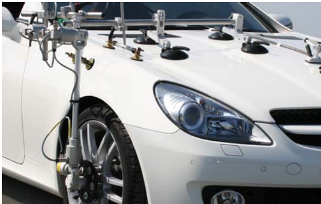
Fig. 4: RV-4 sensor, front wheel mounting with 4-point suction holder
